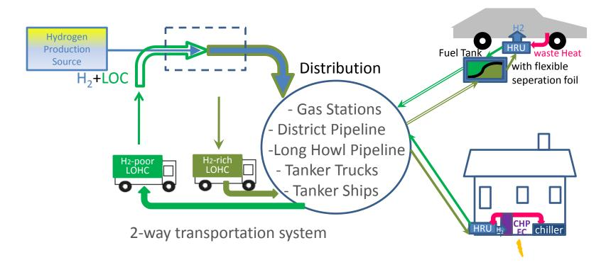
An Integrated Production, Storage and Delivery of Hydrogen – Using Reversible Liquid Carriers
