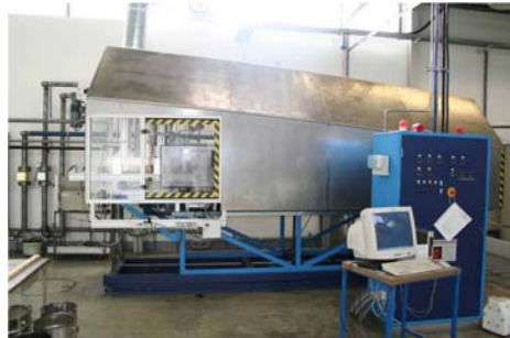
Figure 2 Our catalytic reactor in Austria: C-Polymer (AUT); annual H 2 production: 2 tons/a
