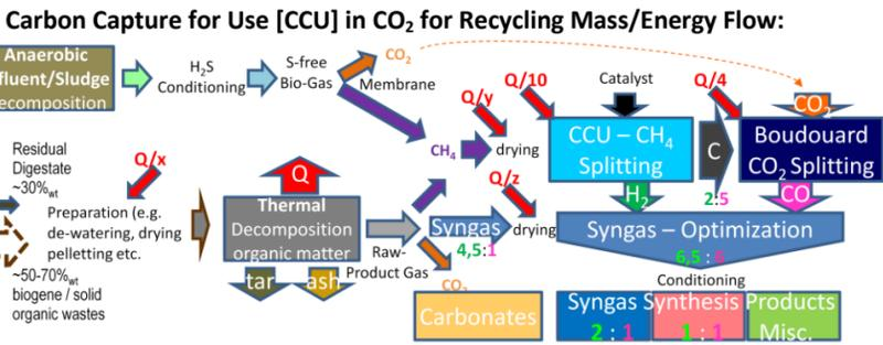
For 2:1 H<sub>2</sub>/CO hydro-carbon synthesis a water-shift reaction can be added, thus allowing flexibility on the final downstream usage paths for the synthesis gas.
