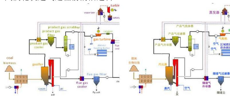
At state of the art gas turbine efficiency in the order of 40% this could generate  $1.6MW_{el}$  in single mode and an additional  $0.8MW_{el}$  in combined heat cycle per ton coal. 根据当前汽轮机效率为40%计算,这将在单一燃烧模式多产生1.6兆瓦电力或在联合热循环中再附加0.8兆瓦电力/**吨煤**
