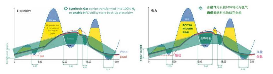
While Photo Voltaic and/or wind energy are productive, the coal gasification plant can in contrast to conventional thermal power plants produce Chemical Synthesis products and therefore achieve economically attractive utilization.
