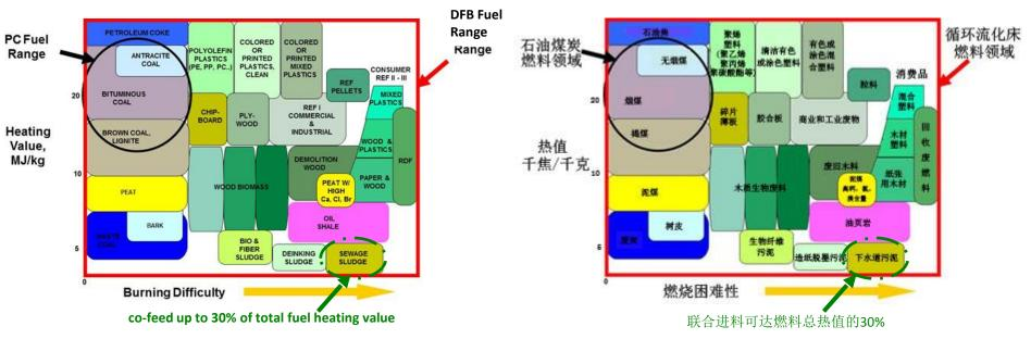
up to 30% of the heating content of fuel could come from renewable or repeatable source 燃料热值的30% 可由可再生和可重复利用资源提供
