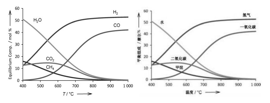
Using steam as a gasification agent allows process adjustments to actual fuel qualities via optimum steam-to-fuel and steam-to-carbon ratios.
