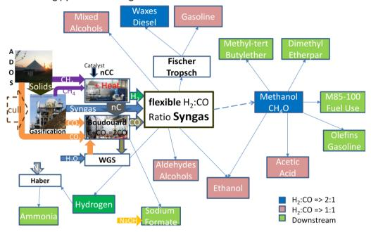
For the example of a downstream FiT-fuel synthesis output the mass-energy flow simulation in IPSE-Pro came out > 40% overall chemical Input/Output energy efficiency, which would outperform the one of fossil fuels.
