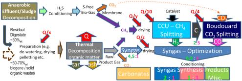
For 2:1  $H_2/CO$  hydro-carbon synthesis a water-shift reaction can be added, thus allowing flexibility on the final downstream usage paths for the synthesis gas.
